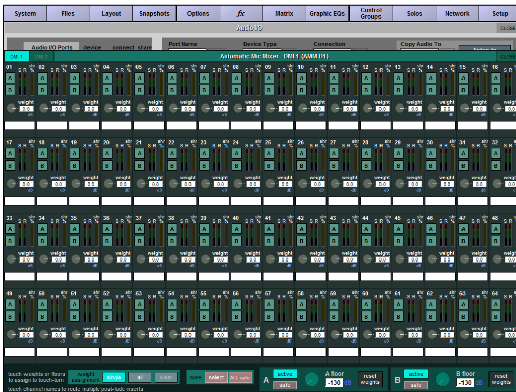
Figure 1: AMM Control Window
